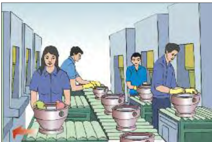
Figure 6d. A passive conveyor line for moving heavy motor castings at working height.
