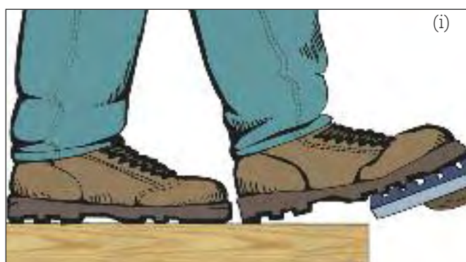
Figure 38a. (i) and (ii) Locate a foot pedal at floor level and make the pedal large enough for easy operation.
