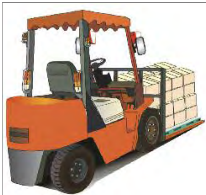
Figure 49a. Provide support to increase the comfort of forklift driving, such as a vibration-absorbing seat, mirrors, overhead structure and appropriate pallets.
