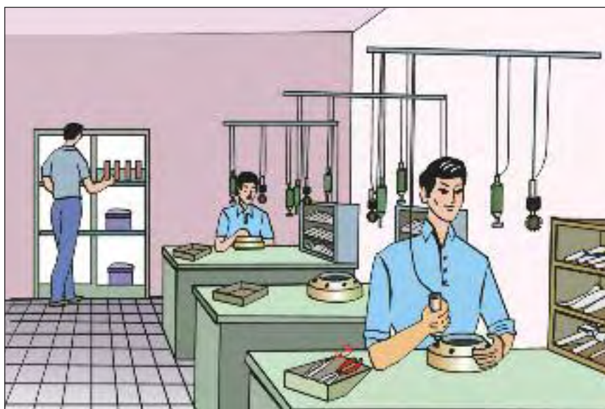
Figure 20d. Placement of tools in accordance with frequency of use.
