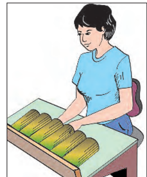
Figure 51b. For seated workers, worksurface height should be around elbow level.
