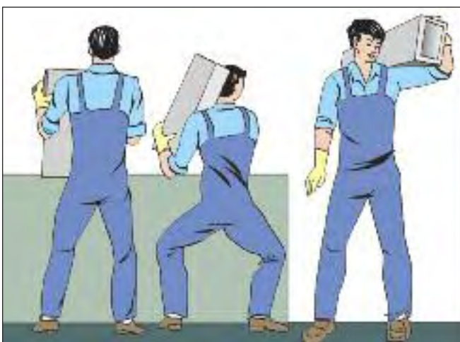
Figure 15b. A long heavy object can be lifted using the power of the legs by keeping the object as close to the body as possible.
