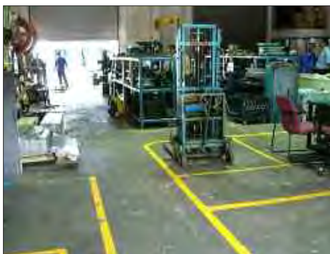
Lines drawn to separate transport routes and storage areas from working areas.
