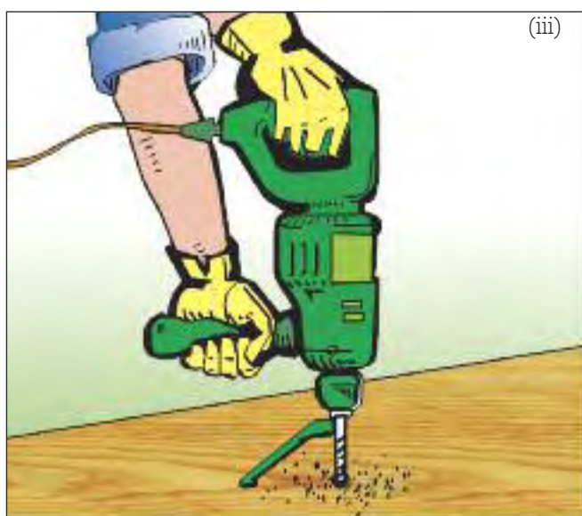
Figure 25. (i), (ii) and (iii) Grips that prevent forward movement of the hand allow safe and effective tool operations.
