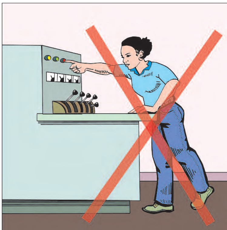
Figure 52b. Avoid a situation where controls or machinery are difficult to reach.
