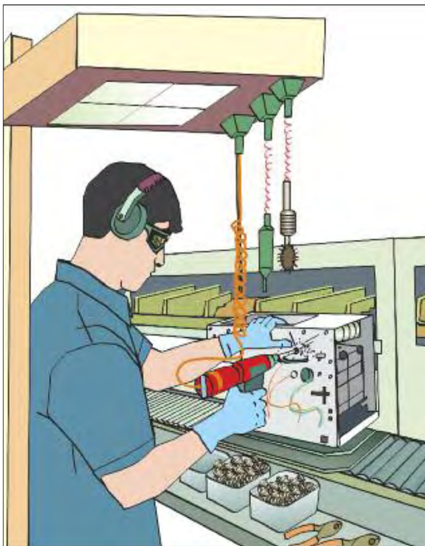
Figure 27. Provide good protection against noise and vibration, such as ear protectors, which protect against the effects of noise, and hand guards, which can diminish the impact of vibration.
