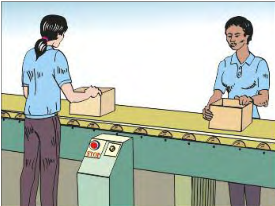
Figure 10c. Reduce manual handling of materials by using conveyers.
