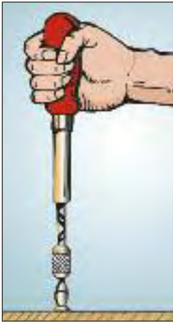
Figure 24a. Alternative tools can be used to reduce mechanical stress, such as a screwdriver equipped with a ratchet.
