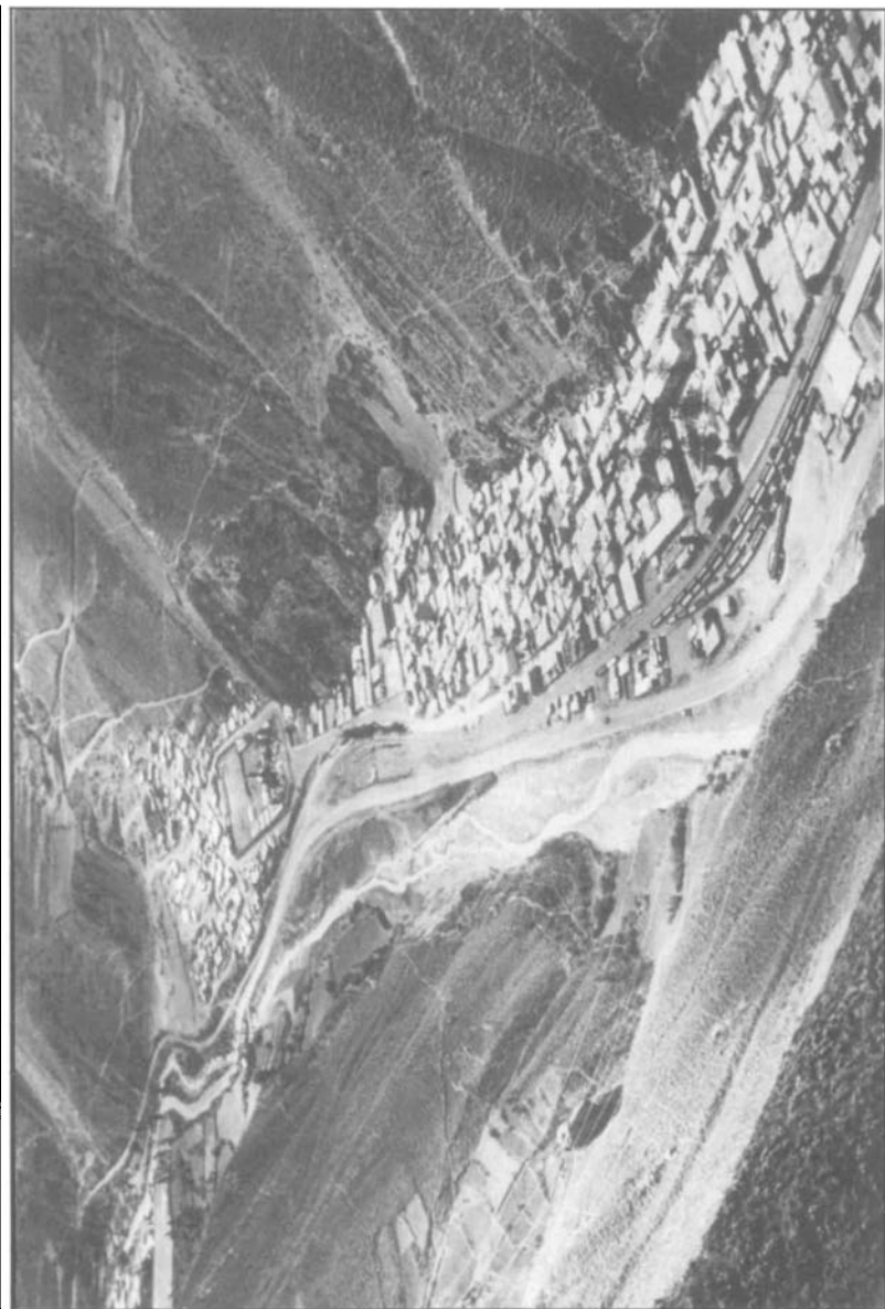
Aerial view of Matucana, Rimac Valley, showing the vulnerable location of the main road, railway and buildings in the floodplain. Erosion is clearly visible on the steep sides of the surrounding mountains, particularly where vegetation cover is denuded.
